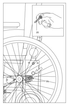
lock the upper holding device [21] with the locking pin [20]. Unlock the locking pin by pushing in its center with your thumb, then drive the locking pin all the way into the holding device.
