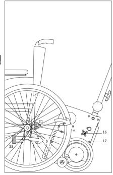
Align all four wheels of the scalamobil in a parallel position by pushing the rocker switch [2] (the device moves downward and the wheelchair sets down on its wheels).
